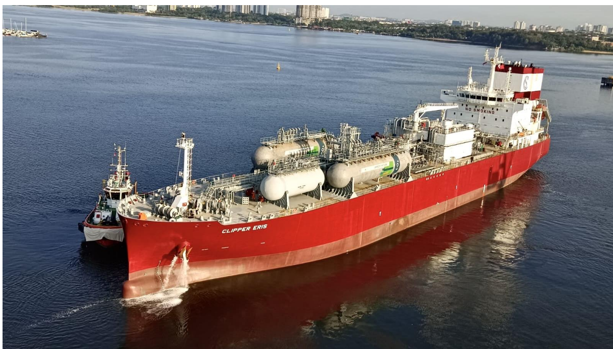
Seatrium proudly delivered Clipper Eris , the world's first full-scale retrofit of a 7MW Carbon Capture & Storage system for Solvang ASA earlier in February this year
